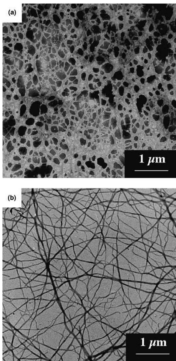
FIG. 1. TEM images of aggregates of (a) (1) and (b) (2) in benzene; initial concentration of (1) (concentration of L-glutamide-derived substituent) = 0.1 unit mM and (2) = 0.1 mM; stained by 2 wt% ammonium molybdate.
