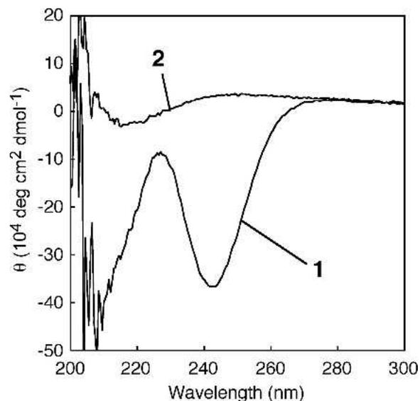
FIG. 2. CD spectra of (1) and (2) in a cyclohexane-ethanol (95:5) solution at 25 °C by using a 1 mm quartz cell. Concentration of L-glutamide moiety, 1.0 unit mM.
