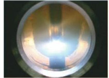
Discharge in supercritical argon
