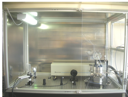
Figure 8. Experimental apparatus of pulsed laser ablation in supercritical CO 2 for material synthesis. (a) Schematic diagram; (b) Photograph.
